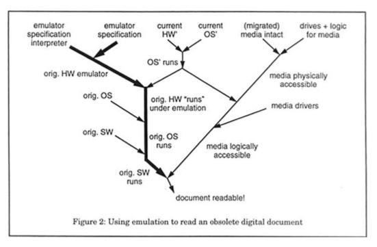
of a readable emulator specification and an interpreter for such specifications allows us to produce an emulator for the original hardware.
